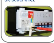
11 Push in the CO wires at the bottom right of the KL08RF for volt-free heating/cooling changeover switching. An open switch is for heating (red LED). A closed switch is for cooling (blue LED).
