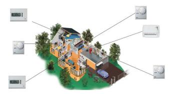
The wireless regulation consists of a transmitter and a receiver. The receiver is available for 1, 2 or 8 zones. The 8 zone receiver uses a connection box to connect the thermo-electric actuators.
